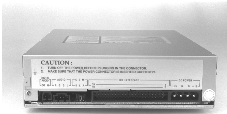
Figure 14.4 The rear connection interfaces of a typical IDE internal CD-ROM drive.
