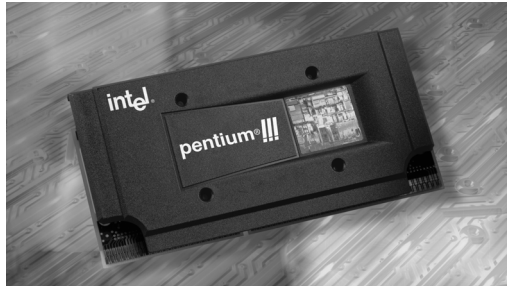
Figure 3.50 Pentium III processor. Photograph used by permission of Intel Corporation.
